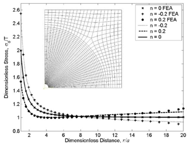
Fig. 1. Verification problem mesh geometry and stress profile comparisons.
