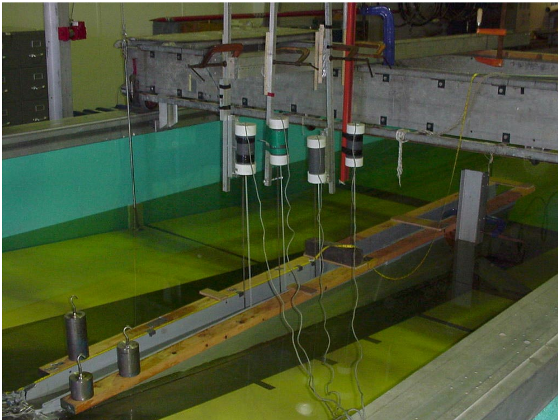
Figure 2: Quasi two-dimensional landslide experiments for benchmark case 2
