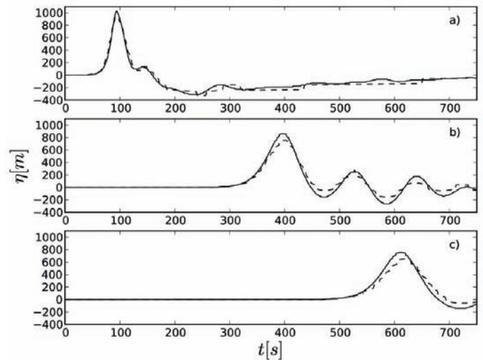
Fig. 4 : Free surface time history (case of Fig. 2) at gage : a) G1 (10 km off-shore), b) G2 (45 km off-shore) and c) G3 (100 km off-shore) for two meshes : mesh 1 (solid line)  $1500 \times 120$  ( $\Delta x = 100$  m, irregular in  $z$ ), mesh 2 (dashed line)  $200 \times 80$  (irregular in  $x$  and regular in  $z$ ).
