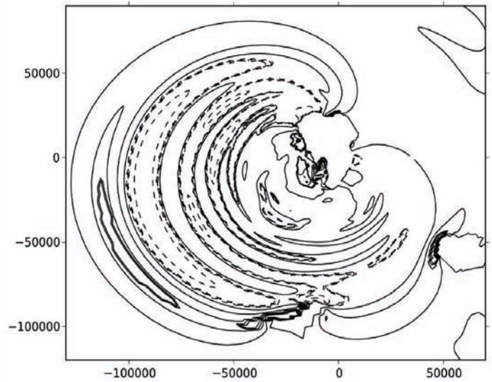
Fig. 10 : Free surface elevation after  $\sim 10$  min ( $t=634 \text{ s}$ ). Contour step equal to 20 m. Positive elevations as solid lines (including 0) and negative elevations as dashed lines. Slide initial volume:  $80 \text{ km}^3$ .
