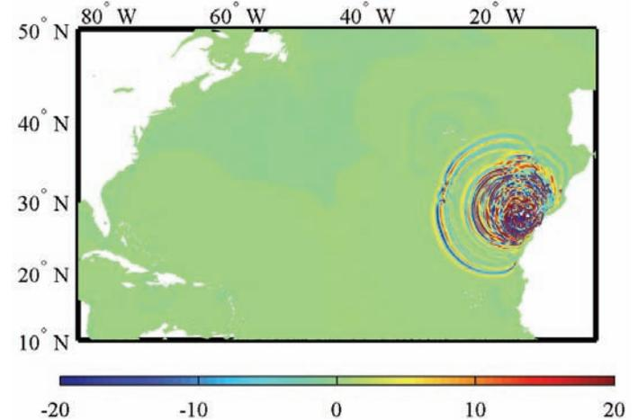
Fig. 16 : FUNWAVE results in the 2' North Atlantic grid, at  $t=93.6$  min. (simulating the first 517 s with THETIS, the next 25 min. with FUNWAVE in the regional 15'' grid, and the final 60 min. with FUNWAVE in the North Atlantic 2' grid).
