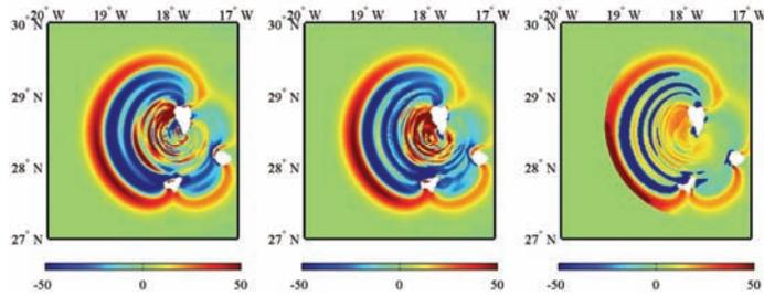
Fig. 14 : FUNWAVE results for surface elevation, for  $t=770$  s, initialized by Thetis results computed at  $t=360$  s (left), 517 s (center), and 770 s (right) (Fig. 12) and interpolated onto the regional FUNWAVE 15 arc-second grid.
