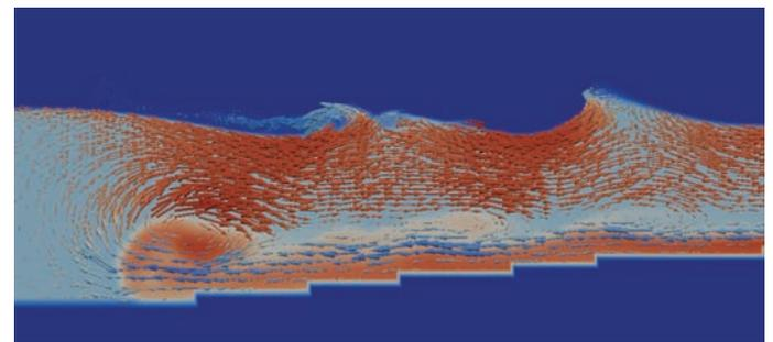
Fig. 8 : Same case as Fig. 6. Detailed velocity field around the slide tip at  $t=438$  s, showing the strong current generated in the water by the slide displacement.
