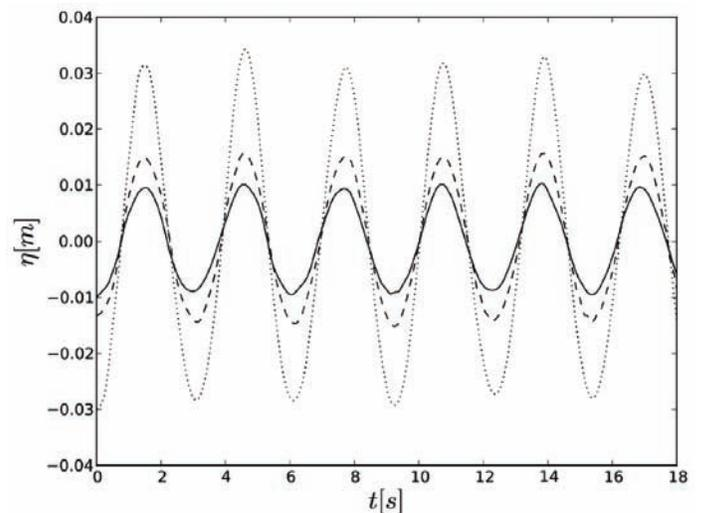
Fig. 5 : linear wave propagation computed with a regular grid mesh ( $\Delta z = 2$  cm). Free surface time history at  $x = 5$  m. Wave amplitudes are: 1 cm (solid line), 1.5 cm (dashed line) and 3 cm (dotted line).
