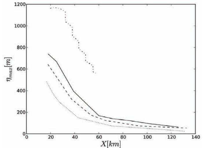
Fig. 11 : Computed decay of the maximum elevation of the first wave for a slide volume equal to :  $20 \text{ km}^3$  (dotted line),  $40 \text{ km}^3$  (dashed line),  $80 \text{ km}^3$  (solid line) and  $450 \text{ km}^3$  (dot-dashed line, run still ongoing).
