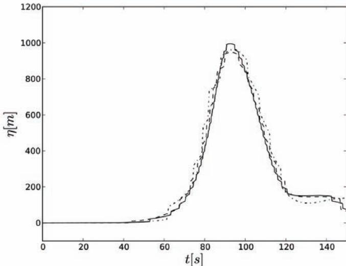
Fig. 3 : Free surface time history (case of Fig. 2) at gage G1 (Fig. 2; 10 km off-shore) for three meshes : mesh 1 (solid line)  $\Delta x = \Delta z = 40$  m, mesh 2 (dashed line)  $\Delta x = \Delta z = 100$  m, mesh 3 (dot-dashed line)  $\Delta x = \Delta z = 200$  m.
