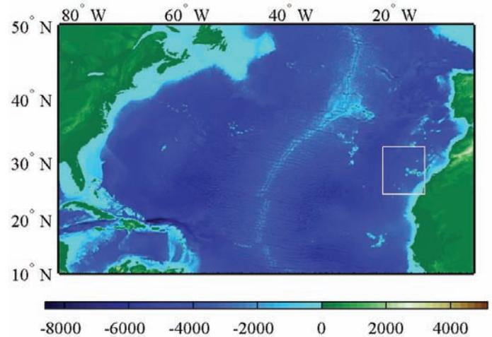
Fig. 13 : Bathymetry of North Atlantic, showing the grid used for trans-Atlantic propagation (2 arc-minute resolution), as well as the smaller, regional grid (white rectangle; 15 arc-second resolution).
