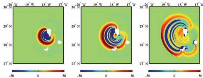
Fig. 12 : THETIS results for surface elevation (color scale in meter) at  $t=360$  s, 517 s, and 770 s (left to right), as interpolated onto the regional, 2 arc-second grid used for FUNWAVE computations.
