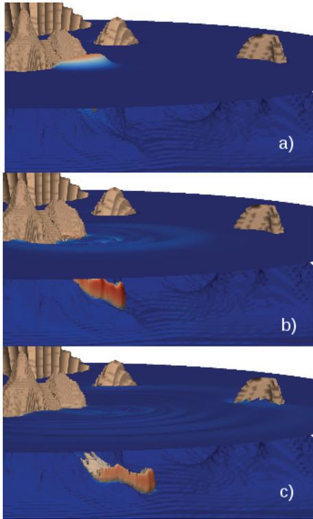
Fig. 9 : Snapshots of water and slide interfaces (volume fractions respectively equal to 0.5 and 0.1) at  $t=$ : a) 2 min, b) 6 min, c) 10 min into the event, with a slide initial volume of  $80 \text{ km}^3$ .
