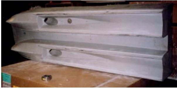
Fig. 5: Picture of 2.3 m long HSC-SES model nearly identical to that used in IMD tow tank tests. Cushion inlets are visible as well as the hole for the acoustic range finder.
