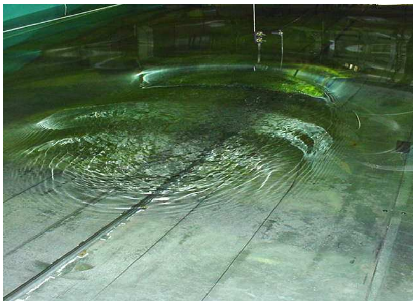
Fig. 2. Example of landslide tsunami generated for d = 80 mm.
