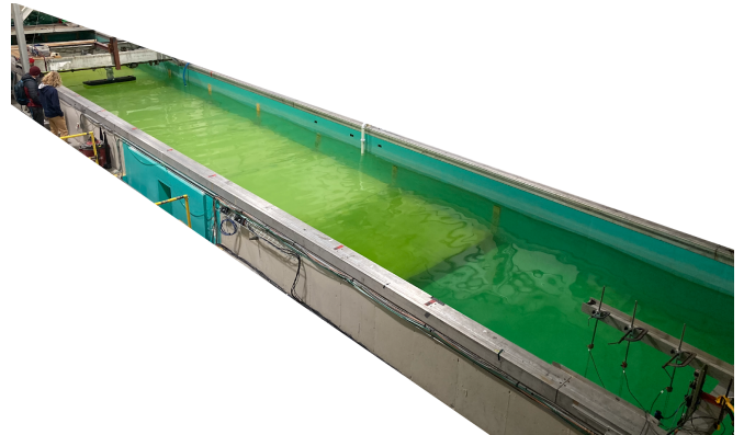
Fig. 2: A view of the entire experimental configuration. Wave gauges placed in the bottom right measure wave elevations and feed them into the NI DAQ. The float can be seen mounted to the carriage in the top left.
