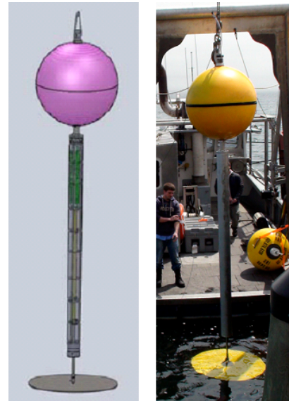
Figure 2. DC2 wave energy buoy; conceptual drawing (left) and 1:4 scale prototype (right)
