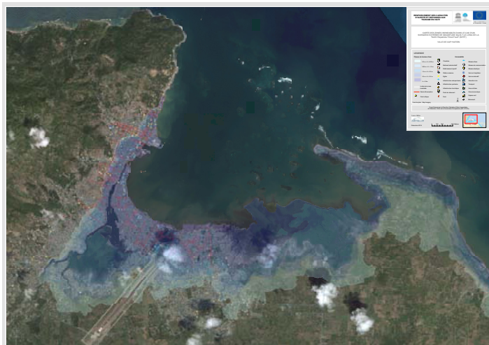
Fig. 13: Maximum flow depth computed with TELEMAC around Cap Haitien, in 12-30 m resolution irregular FEM grid (footprint of the grid is also shown in Fig. 2b), for the M_w 8.7 near-field seismic NHTF source.
