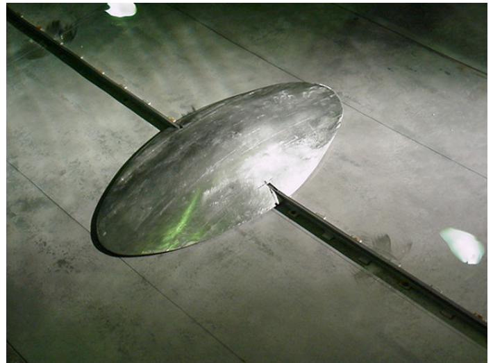
Fig. 2: Landslide resting on top of the guiding rail
